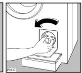
Unscrew and remove the filter.
